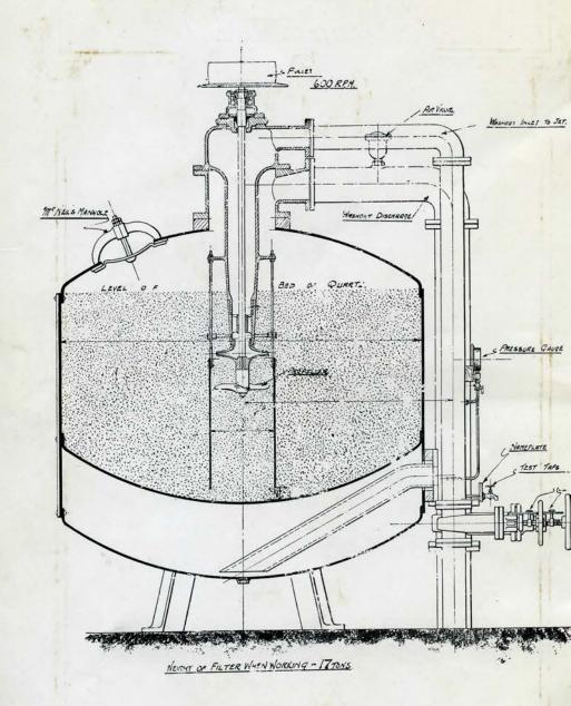
Sectional View of 8ft. diameter Filter
